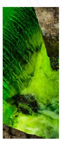
In practice, the quantity is expertly estimated, taking into account the hydrogeological context. Between empiricism, intuition and experience, to decide the question, two determining elements must be taken into account: the dilution that the tracer should undergo, often approached by means of distance and the analytical performance of the tracer, and the monitoring modes.
