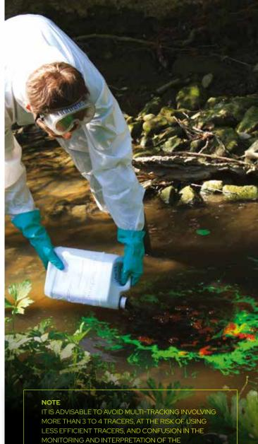
MORE THAN 3 TO 4 TRACERS, AT THE RISK OF USING LESS EFFICIENT TRACERS, AND CONFUSION IN THE MONITORING AND INTERPRETATION OF THE RESTITUTION CURVE(S):
