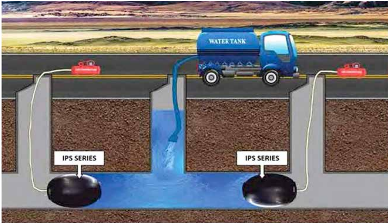
Picture-1 IPS series in pipeline water filling testing
